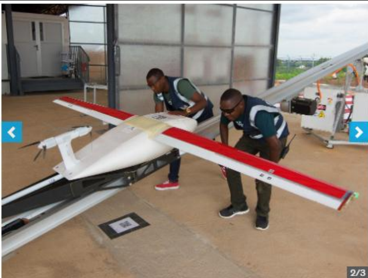
Next they place the drone on the catapult and run through preflight checks to prep the aircraft for launch. Photo: Evan Ackerman
