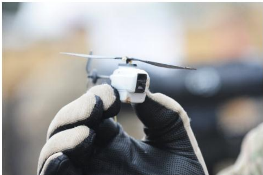
A PD-100 in a soldier's hand, showing the front camera.
