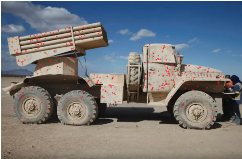
Figure 4.3 GMLRS Alternative Warhead Effects on BM-21 Test Target
