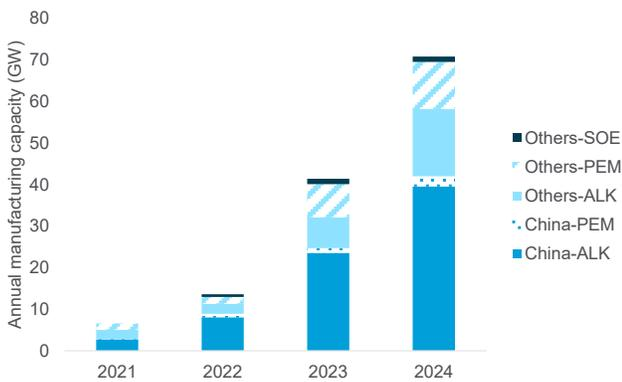
Note: ALK refers to Alkaline Electrolyzer, SOE refers to Solid-Oxide Electrolyzer. Source: BNEF, Citi GPS
