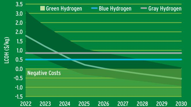
Note: Assuming natural gas price of \$3/MMBtu. Green hydrogen is powered with dedicated solar power. LCOH=levelized cost of hydrogen.
