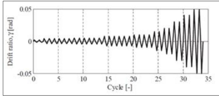
**Figure 7** Seismic Loading Protocol in the Validation Model [1]
