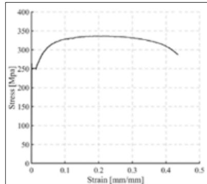
**Figure 5** Stress-Strain Curve of the ASTM-A370-17 Material Used in the Validation Section [1]
