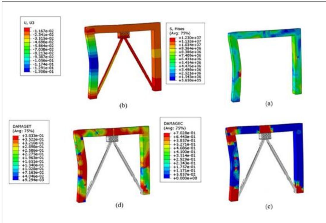
(a) Stress Distribution Contour (b) Displacement Distribution Contour (c) Compressive Damage Contour in Concrete (d) Tensile Damage Contour in Concrete.
