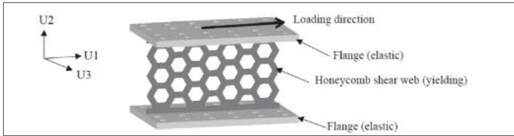
**Figure 2** The proposed honeycomb nest bee damper in the study by Yang and colleagues [1]
