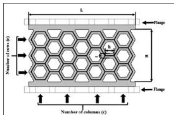
**Figure 3** Geometry and Parameters of the Honeycomb Nest Bee Damper [1]
