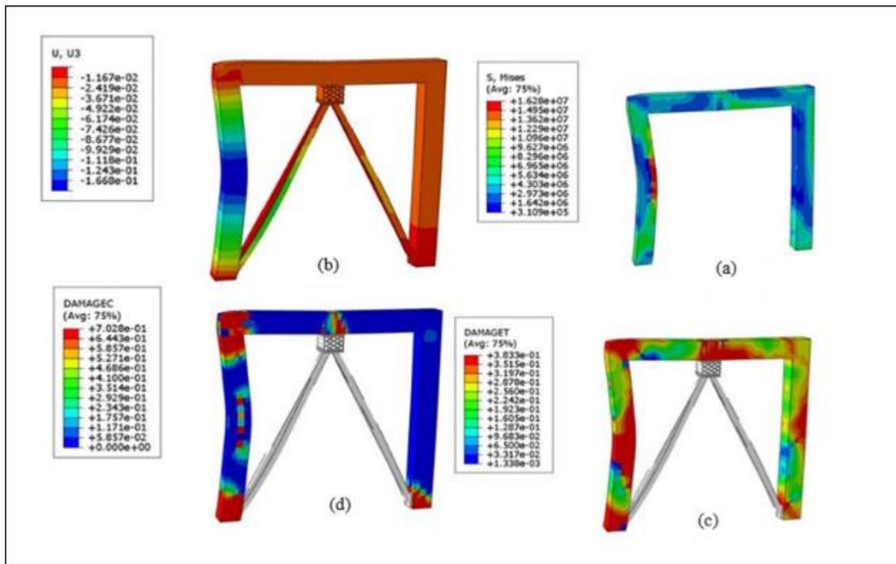
(a) Stress Distribution Contour. (b) Displacement Distribution Contour. (c) Tensile Damage Contour in Concrete. (d) Compressive Damage Contour in Concrete
