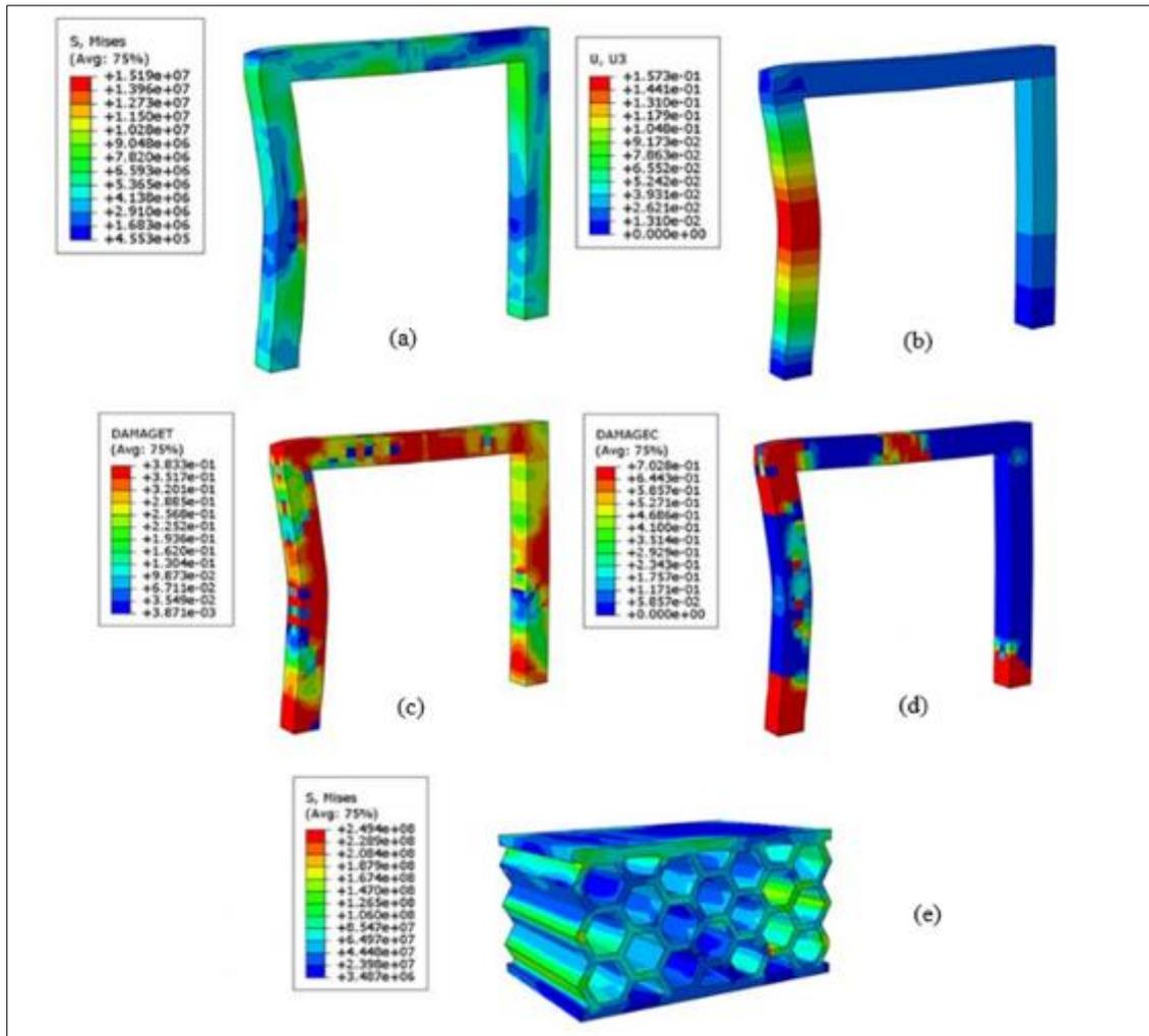
(a) Stress distribution contour. (b) Displacement distribution contour. (c) Tensile damage contour in concrete. (d) Compressive damage contour in concrete. (e) Stress distribution contour in the honeycomb cells
