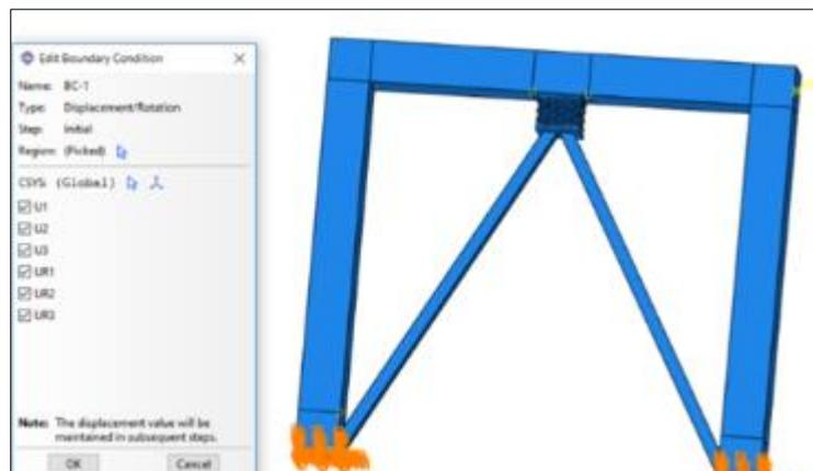
**Figure 11** Restraint of Concrete Column Bases
