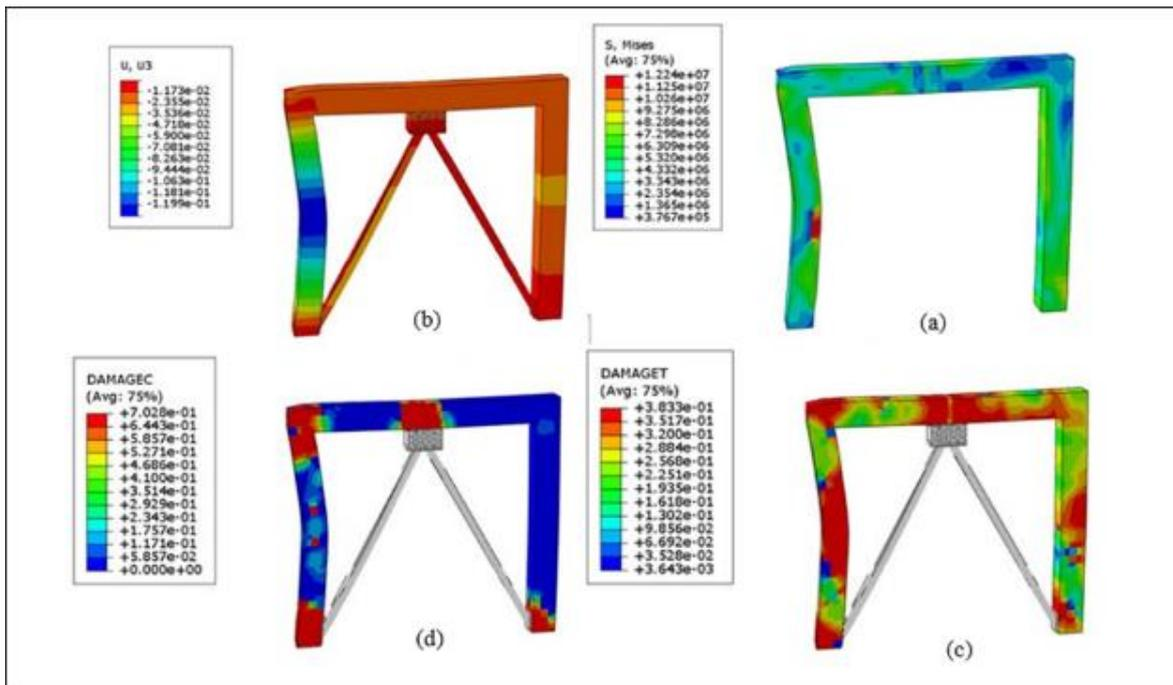
(a) Stress Distribution Contour. (b) Displacement Distribution Contour. (c) Tensile Damage Contour in Concrete. (d) Compressive Damage Contour in Concrete.
