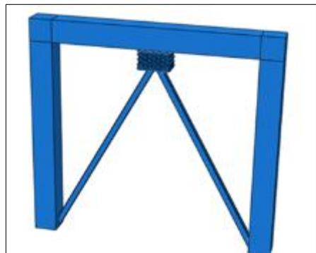
**Figure 1** The Wasp Nest Damper Used in the Proposed Concrete Structure in this Study
