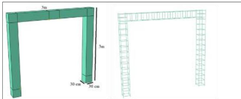
**Figure 10** Geometry of the Concrete Section and Reinforcement Details Used in the Models
