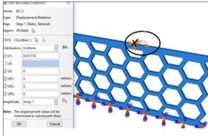
**Figure 8** Location of Seismic Loading Application
