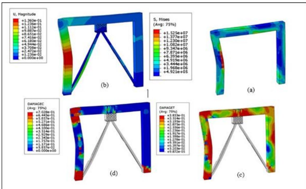
(a) Stress Distribution Contour. (b) Displacement Distribution Contour. (c) Tensile Damage Contour in Concrete. (d) Compressive Damage Contour in Concrete.
