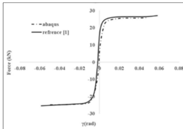
**Figure 13** Comparison of Hysteretic Response Curves Obtained from Abaqus Analysis and the Reference Article [1]
