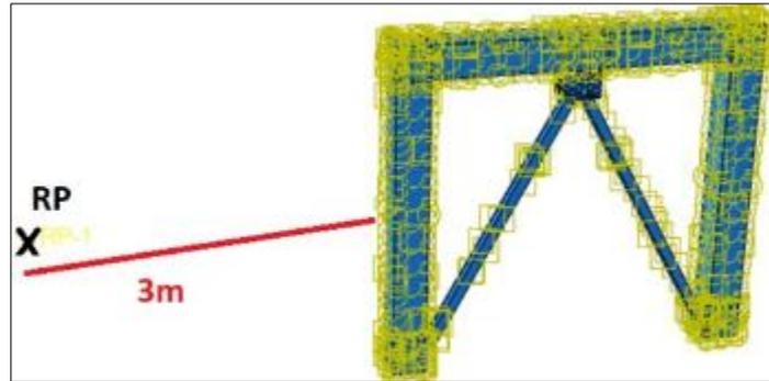
**Figure 12** Distance and Location of Explosive Load from the Structure
