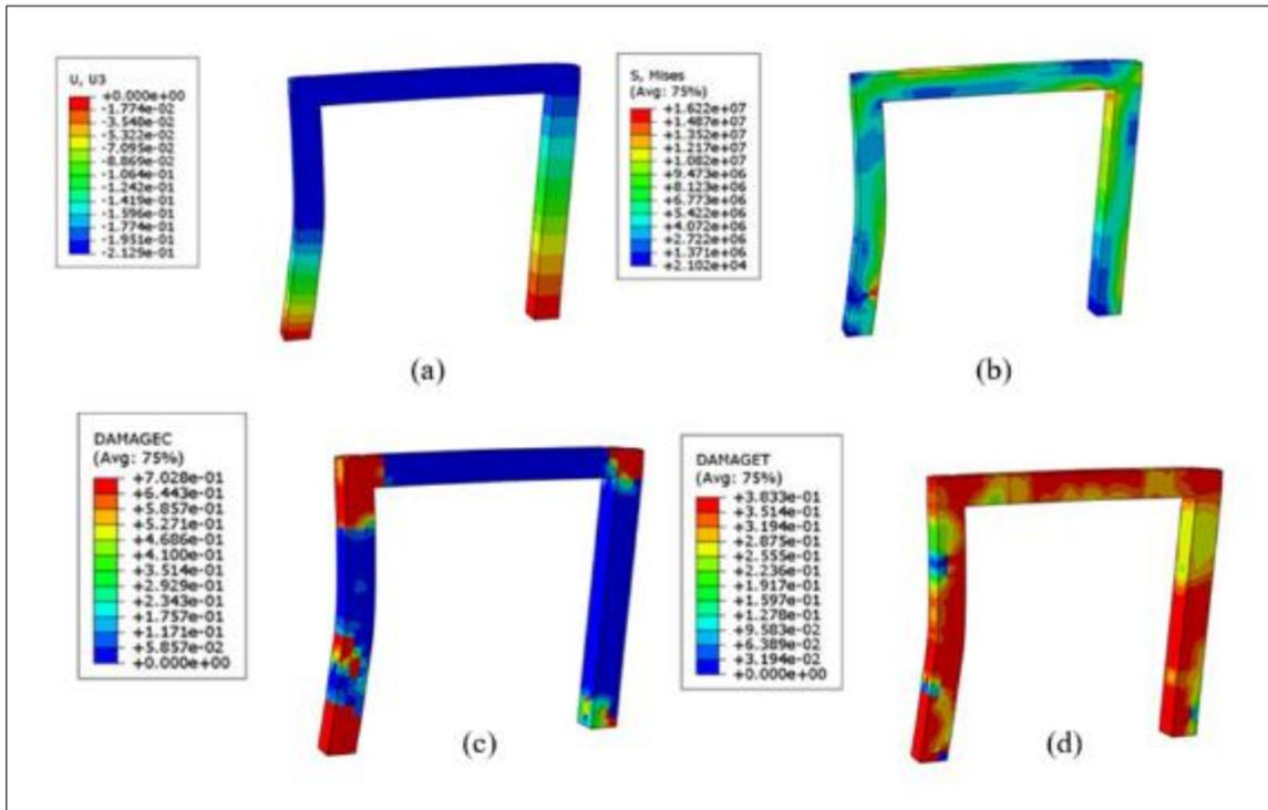
(a) Displacement Contours. (b) Stress Distribution Contours. (c) Compressive Damage Contours in Concrete. (d) Tensile Damage Contours in Concrete
