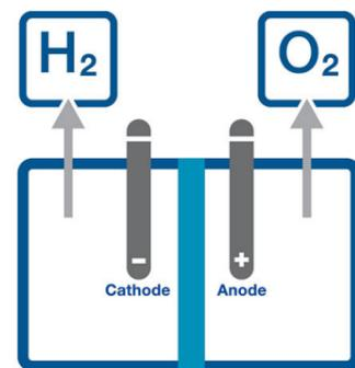
**FIG. 7.** A H<sub>2</sub> electrolyzer separates water into H<sub>2</sub> and oxygen molecules using electricity.
