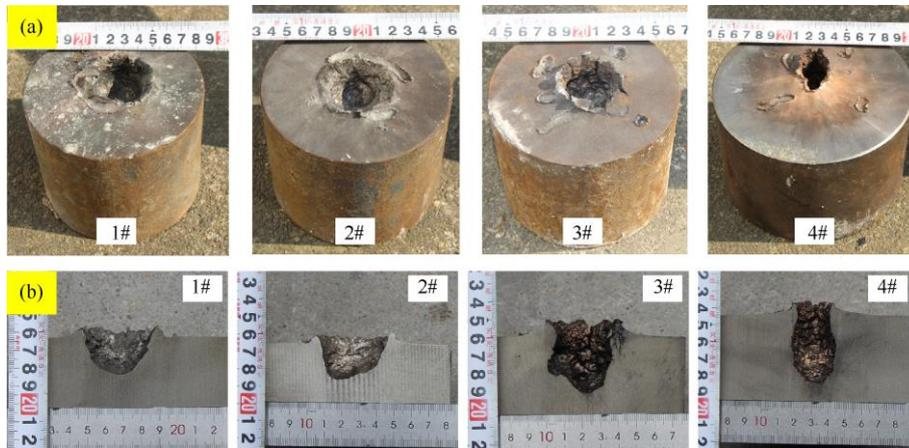
Fig. 7. The damaged steel plates: (a) Entrance hole morphology; (b) Sectional views of
