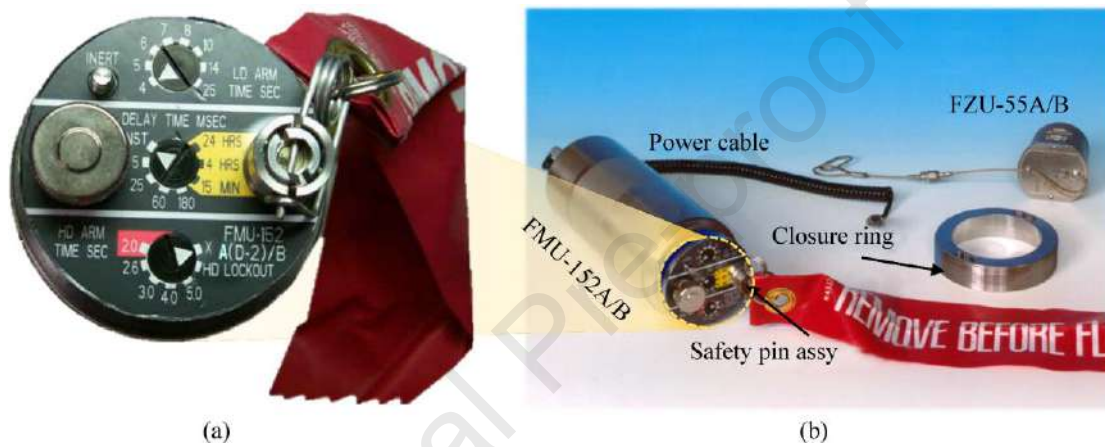
Fig. 7. FMU-152A/B: (a) Close-up view of the manual setting panel [28, 94]; (b) The fuze and components [94].
